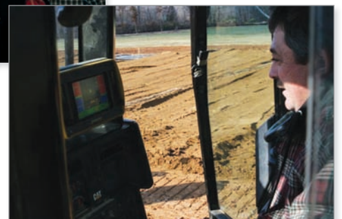
Ronald Franks Construction Equipment Operator Ricky Cooper uses Topcon GPS equipment to assist him in making more efficient passes in forming the Reedy Creek Dam embankment.
